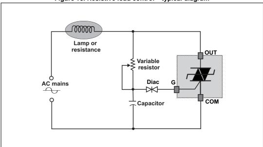
Figure 18. Resistive load control – typical diagram
