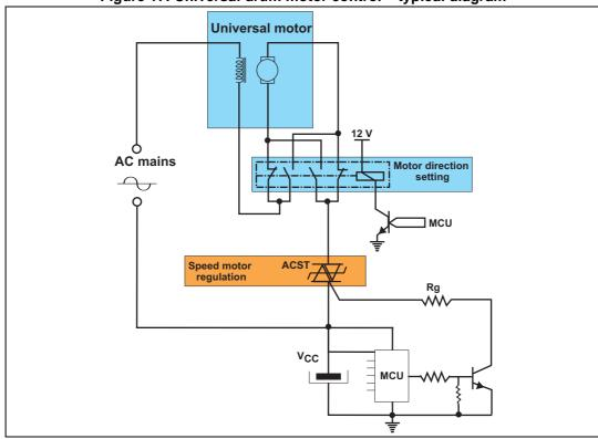
Figure 17. Universal drum motor control – typical diagram
