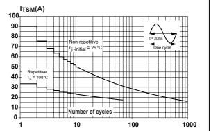
Figure 8. Non repetitive surge peak on-state current for a sinusoidal pulse with width tp < 10 ms, and corresponding value of I<sup>2</sup>
